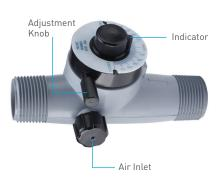
The Pentair® Wellmate® Micronizer installs easily to any hydropneumatic tank, drawing air into the water line through the air inlet. When properly installed and adjusted, the Wellmate Micronizer by Pentair will continually charge the tank with air for 30% to 50% of the pump's run time. Excess air is relieved through an Air Volume Control assembly installed in the tank.
